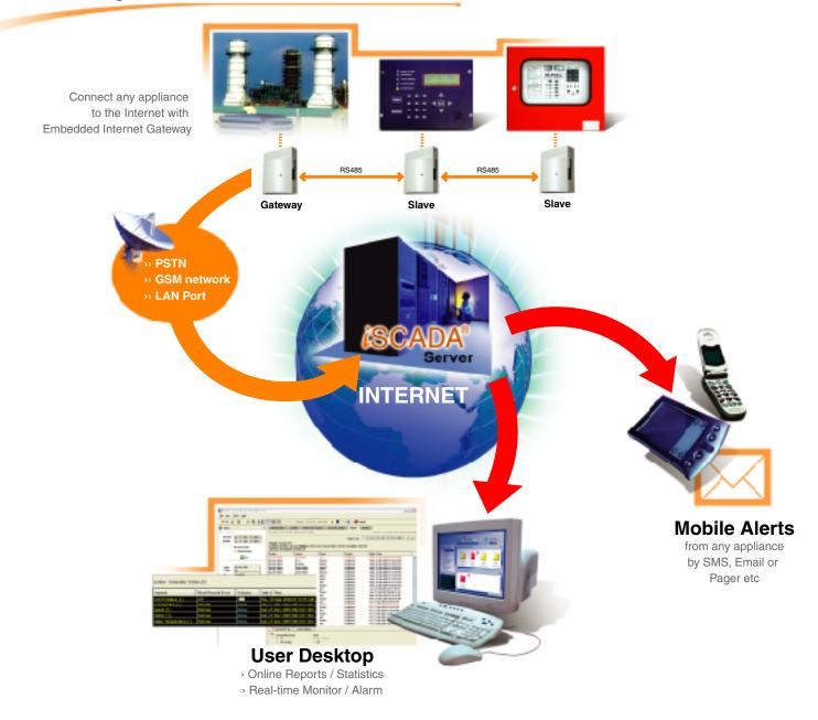
Any existing appliance can be easily Internet-enabled by retrofitting an **iSCADA** Gateway, which is a compact low cost device that gathers information from your appliance and transmits them to the **iSCADA** server. Users may monitor and control their appliances remotely from any Internet connection using only a browser.
